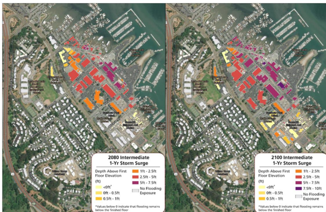
Figure 10 Flood Depth Above First Floor Elevation (ft) for 2080 Intermediate Scenario, 1-year Storm Surge (Left), and 2100 Intermediate Scenario, 1-year Storm Surge (Right).
