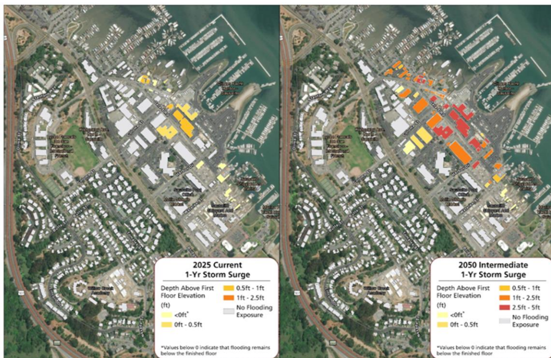
Figure 9 Flood Depth Above First Floor Elevation (ft) for 2025 1-year Storm Surge (Left), and 2050 Intermediate Scenario, 1-year Storm Surge (Right).
