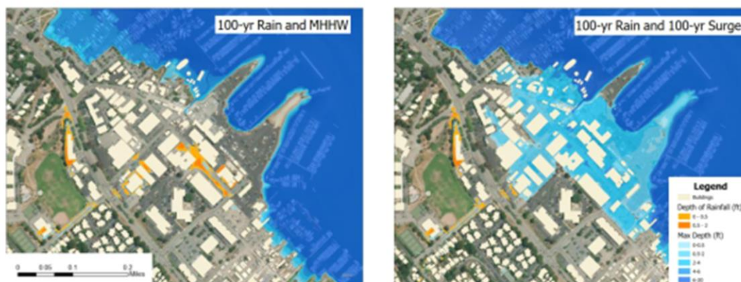
Figure 4 Rainfall Driven Flooding Versus Tidal Driven Flooding in the 2025-Time Horizon.
